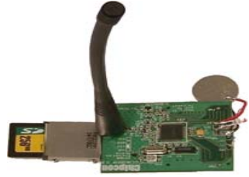
Fig. 1. a) Soil-Organism Monitoring Application: Each sensor stores locally on external flash memory the CO_2 levels in a sliding window fashion. The user might then ask: "Find the time instance on which we had the highest average CO_2 levels in the last month?". b) Our platform: The RISE (Riverside Sensor), which is the first sensor device that features a large external storage medium (an SDMedia flash card) .
